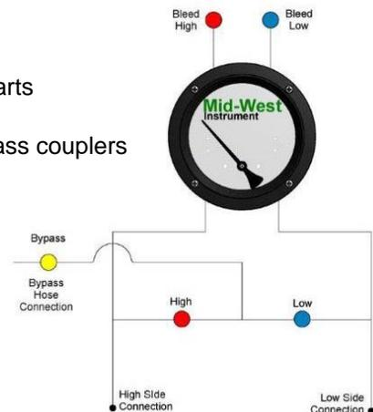
Gauge is capable of performing all known test procedures including those recommended by ABPA, ASSE, AWWA, CSA, FCCC and HR-USC, NEWWA and UF-TREEO
