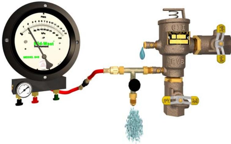
The 830-0001 has a soft seated needle valve, a quick coupler for connection to a ¼” flare fitting at the test cock and a flare connection for connection of the test kit hose to the assembly.
